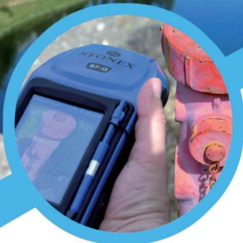
Wi-Fi, Bluetooth, 3G modem, 5 MP camera, voice call and MMS, Mini waterproof USB connector
